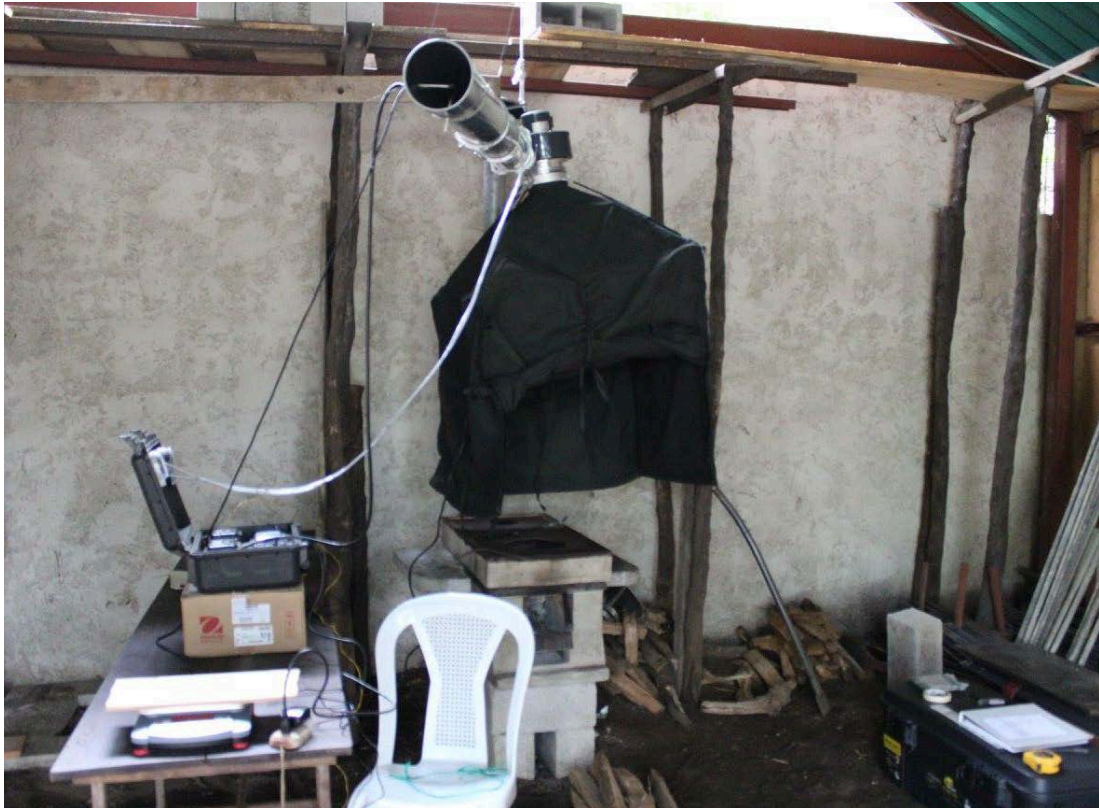
Figure 3. PEMS setup above EcoPlancha
